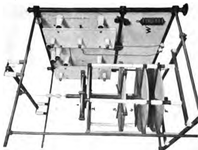
FIG. 142 b .—Back of aerial lengthening coil panel (15 T. K.). [To face p. 281.]
